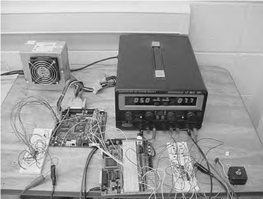
Figure 12. Experimental setup of prototype temperature controller with test equipment.
